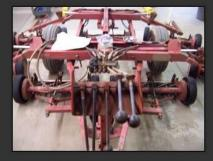
I started the search for the valve on the internet. I found the Cross Company out of Greensboro, NC. They are a distributor for Walvoil valves. After talking to Walvoil we decide the valve we needed was model 18ES3(X5)/RC-SAE-12vdc. The valve came complete with solenoids. There is a solenoid on each side of the spool to make it bidirectional. I also ordered the Canfield
