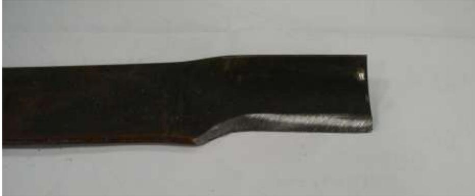
You can avoid producing a hook grind or a step grind by grinding the blend radius into the blade...
