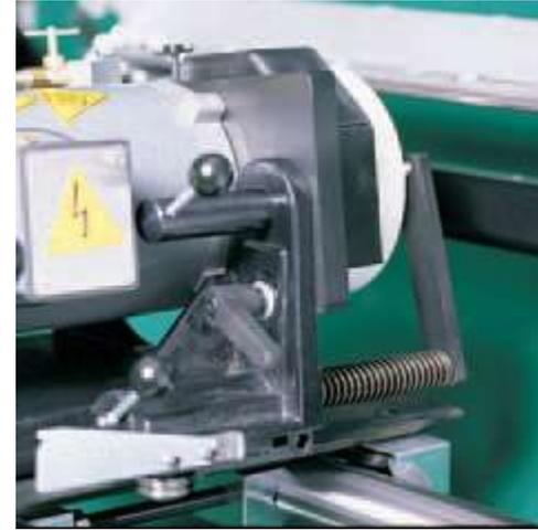
This picture shows the diamond dresser released and in a stroke position to face the stone...
