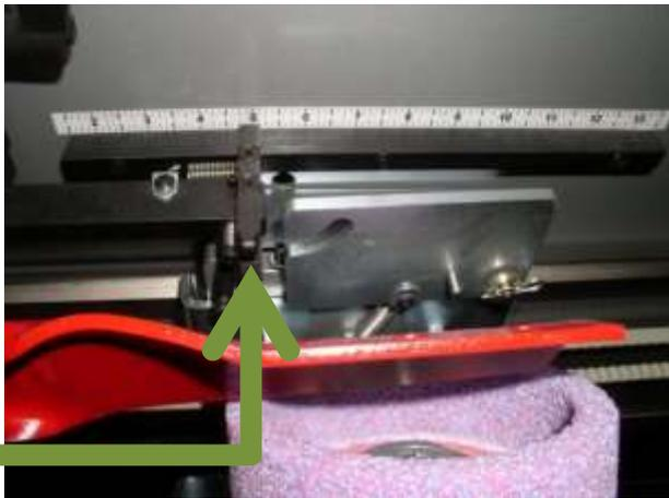
The blend is created by a tilting radius bar...
