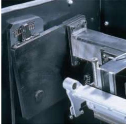
All angles specified by the Reel Manufacturer is in relation to the bottom surface of the bedknife. Mounting has been made much easier by use of magnetic surfaces .
