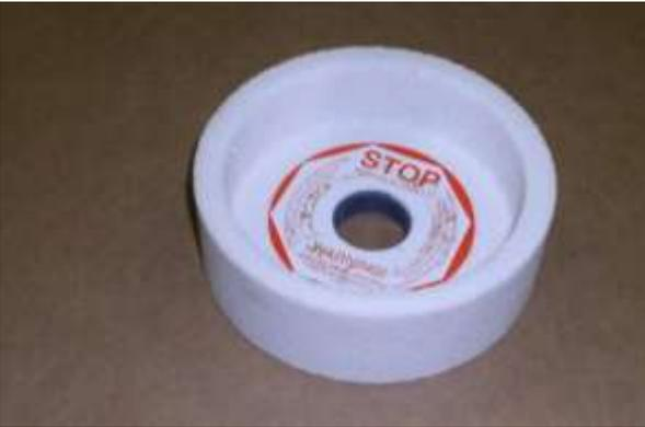
**Standard Cup Wheel:** This is a “vitrified” ceramic based stone that is designed for low impact grinding and is formulated of Silicone Carbide with a ceramic binder. These wheel need to be dressed using a diamond dresser. Dressing the wheel removes imbedded material from the face of the wheel, exposes new sharp cutting edges on the grit, and relieves the ceramic from between the grit stones making it grind more aggressively.
