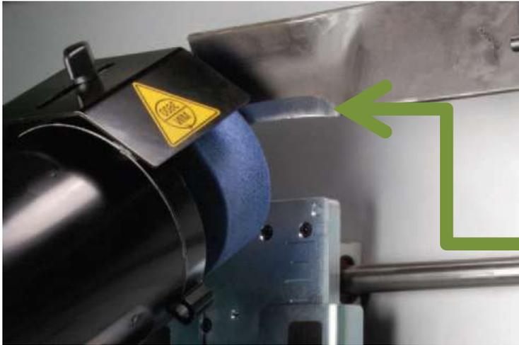
The picture on the left illustrates the ground area and a very distinct blend radius that is built into the blade. This “blend” radius minimizes stress points in the blade as it’s ground through its life.
