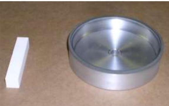
**Borazon Cup Wheel:** This is an aluminum cup wheel that has a borazon coating imbedded on the rim area. Borazon is a super abrasive compound. The “dressing” process is different than what is used on ceramic wheels. This stone comes with a hand held dressing brick that is formulated to clean the surface without removing borazon material. This will keep the wheel free cutting without loading up.
