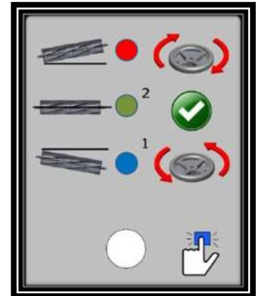
There are new gauging systems that are visual, and tells the operator which way to turn the handle for proper alignment.
