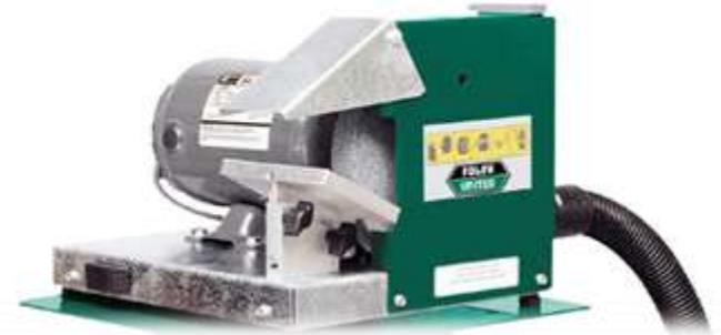
The cutting edge angle should be approximately 30 (thirty) degrees. If it is not, adjust the blade guide and/or the depth control until the desired bevel is achieved.
