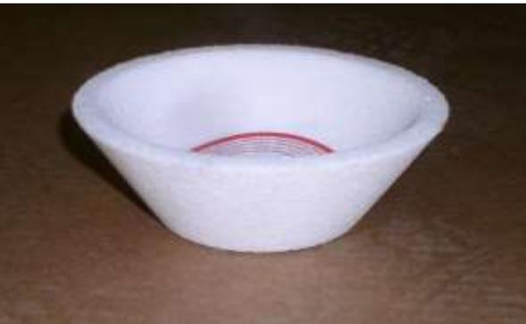
**Flared Cup Wheel:** This wheel is the same composition as the standard cup wheel, but is flared to provide more clearance with obstructions that may exist on certain bedbar shoes. This wheel is also dressed with a diamond dresser. All vitrified wheels need to be checked for cracks before mounting by a practice called “ringing”.
